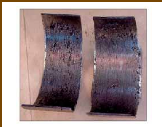
Figure 12. Deformed pieces of steel bearing backing.
