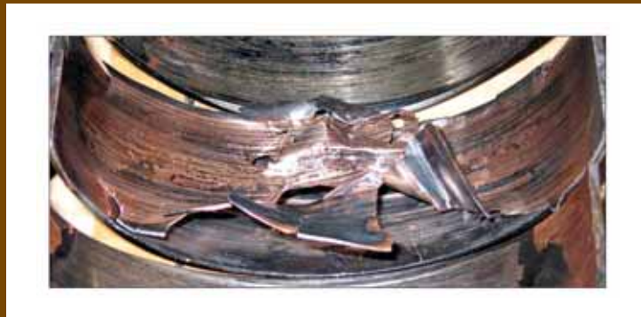
Figure 12. Deformed pieces of steel bearing backing.
